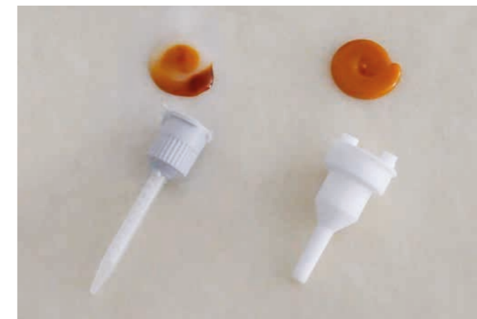
Comparison: Comparison: Mixing result static mixing (le), mixing result Mixing result eco-DUOMIX (dynamic mixing) dynamic
