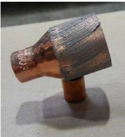
Soldering paste application manual vs. eco-SPRAY
