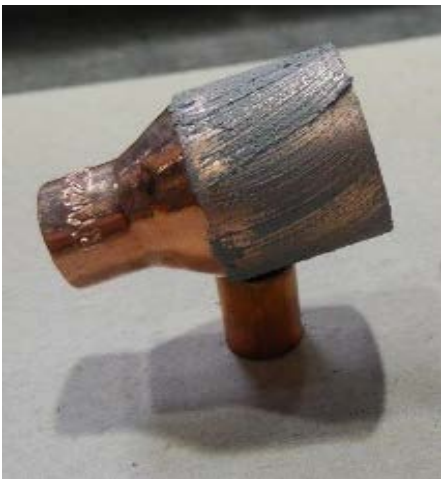
Lotpastenapplikation manuell vs. eco-SPRAY
