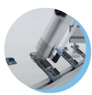
min. dosing quantity 50 μl volume flow 0.5 to 6.0 ml/min weight approx. 640 g
